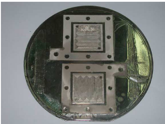
Fig. 11. First layer electroforming of main flow field channel.
