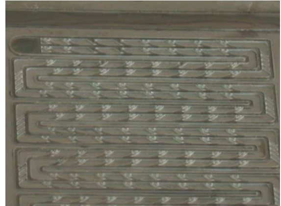
Fig. 12. Second layer electroforming of micro-features.
